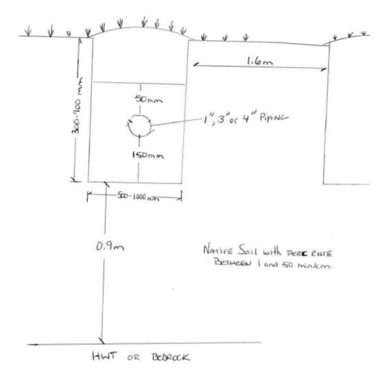
This is an example of a Class 4 Trench Bed cross section depicting one of several runs and its corresponding depths.
