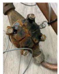
This picture shows the underside of a water meter removed from a building that was unheated during the winter months. The frost plate of the meter is cracked from the water in the meter having frozen and expanded.
